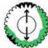
AS A HEAVY SPOT GOES UP, THE FLUID IS FORCED DOWN TO A LIGHT SPOT
