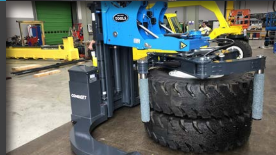
Precise 90° tilt, horizontal to vertical
