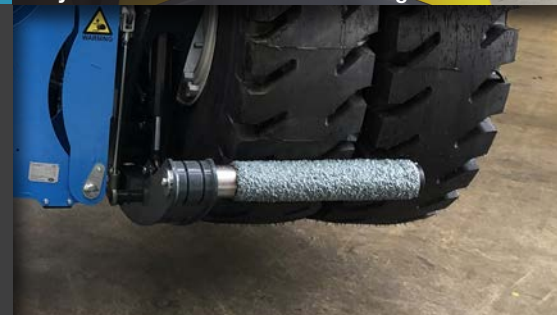
Stone-coated pipes ensure a safe grip
