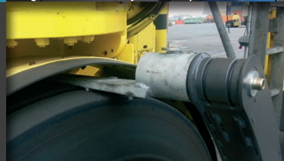
Flat top arm for limited tyre clearance
