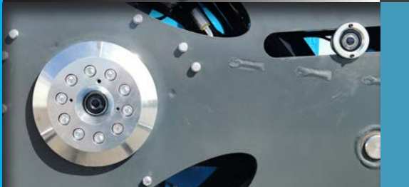
2 Camera System - for hub and bolt alignment
