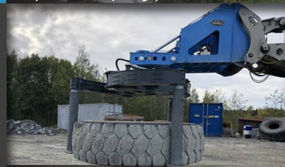
35° or 90° tilt module - horizontal to vertical
