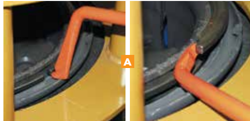
Pry-out end reaches behind slotted end of split ring to pry it out and over the flange of the wheel
