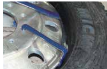
CURVED END For mounting and demounting top bead
