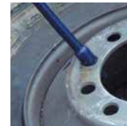
Specially designed forged knob end for hub side up
