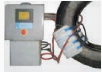
Section Repair Molds
