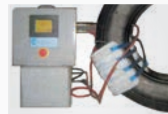
Section Repair Molds
