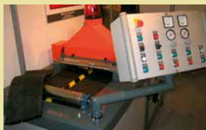
Control panel mounted on moveable arm / Panel de control con brazo pivotante
