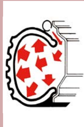
Principle of the Omega Bead Seater
